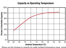
$\label{eq:monotone} \textbf{Amoient lemperature (°C)} \\ Shown are the changes in capacity for wider ambient temperature range, giving the available capacity, as a percentage of the rated capacity, at different ambient temperatures.$
